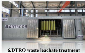
6. DTRO waste leachate treatment equipment
